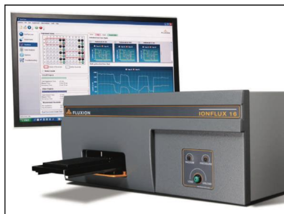
Figure 1: The IonFlux system utilizes a “plate reader” format to simplify workflow and increase throughput. Systems are available with 16 and 64 amplifiers. Throughputs of 10,000 data points per day can be achieved.
