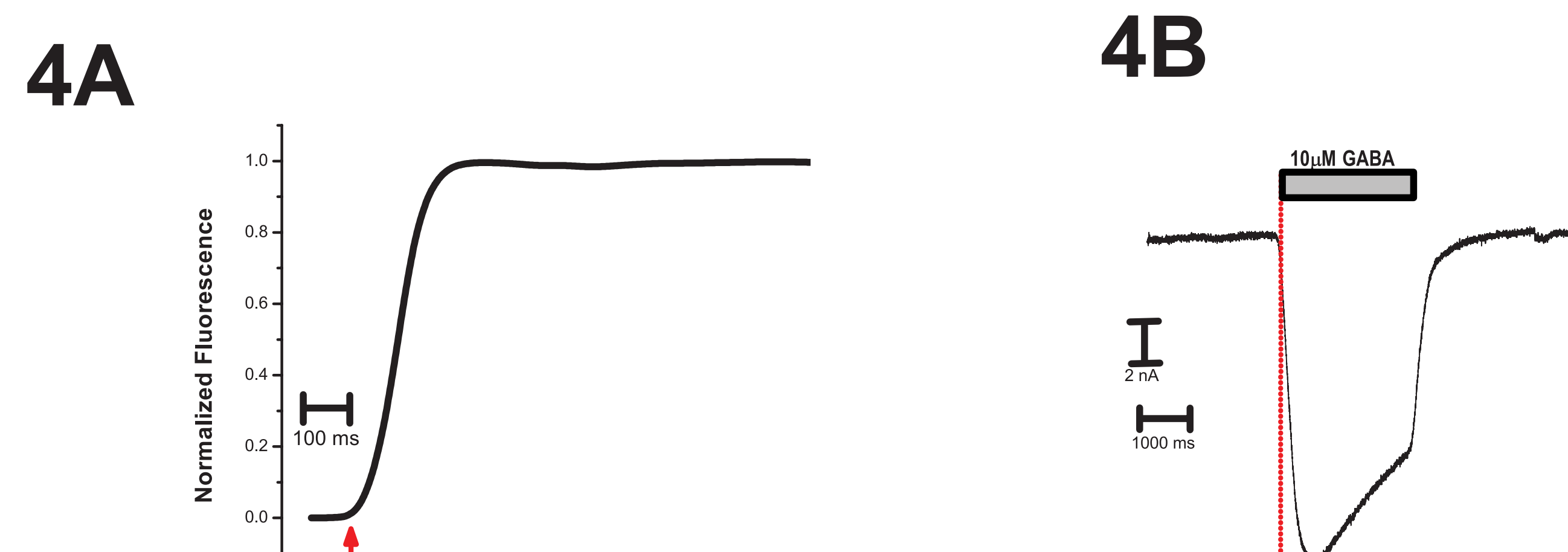
Figure 4. Rapid Compound Application. Figure 4A shows the rapid time course of compound application measured with the fluorescent dye calcein. The red arrow indicates the start of compound application. There was rapid exchange of solution from 0 to 90% in 100 ms. Figure 4B shows an inward Cl - current during exposure of 10 µM GABA to an ensemble of HEK cells expressing hGABA A receptor/channels. Maximum current was recorded within 400 ms in agreement with known GABA A current rise-time.
