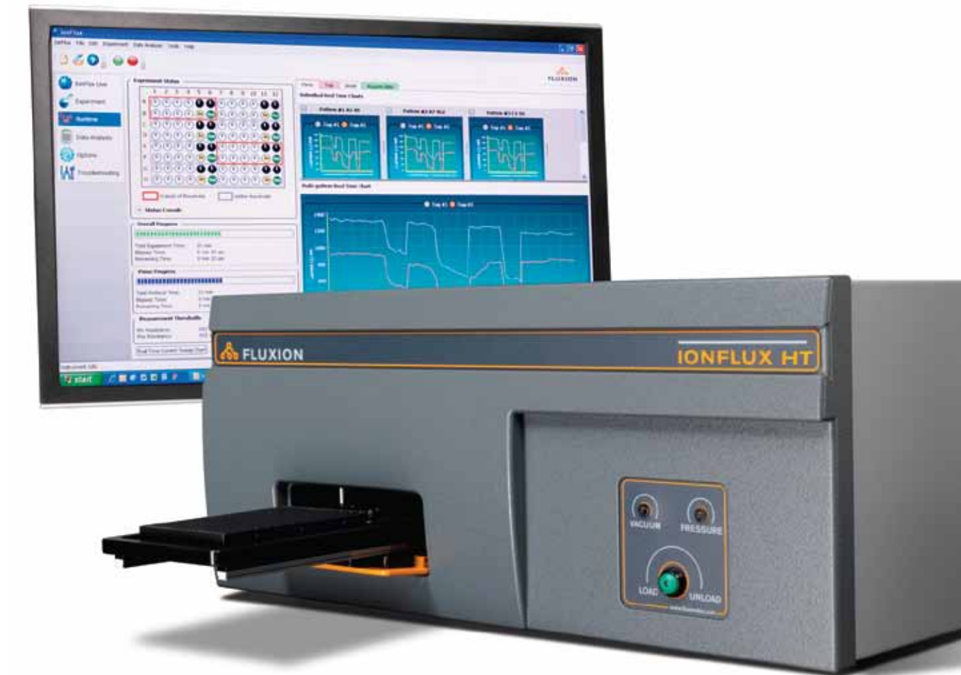
Figure 1. The IonFlux system is designed to operate much like a plate reader. The entire recording protocol, including cell trapping, whole cell formation, compound perfusion, and ion channel recording is managed automatically via software. Plates are preloaded with cells, compounds, and reagents using conventional liquid handlers. Once filled, plates are fed automatically into the IonFlux system. All fluidic control necessary to trap cells and deliver compounds is handled within the instrument, and integrated electrodes record currents.
